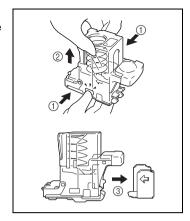
6 (Finisher F-8430) Insert the new staple cartridge into the staple holder, and then carefully remove the stopper.
